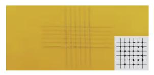
■ ISO Class.: 1 / ASTM Class.: 4 B Detachment of small flakes of the coating at the intersections of the cuts. A cross-cut area not significantly greater than 5 % is affected.
