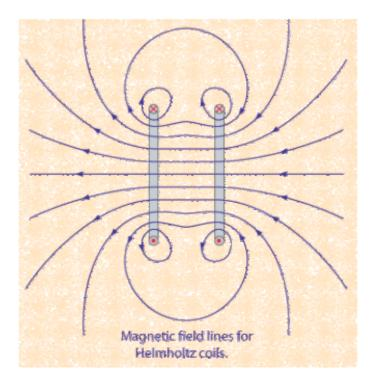
This was the original purpose of the Helmholtz coil to create a very homogeneous magnetic field inside two separate coils. The coils would have a certain radius, and as long as they 2 coils were then separated by this exact same radius, then the magnetic field inside the 2/3 of the coils radius there was a perfect homogeneous magnetic field.
